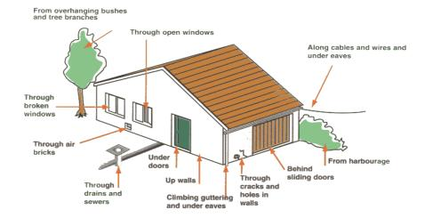
Figure 1: Potential rodent access routes into a building.
